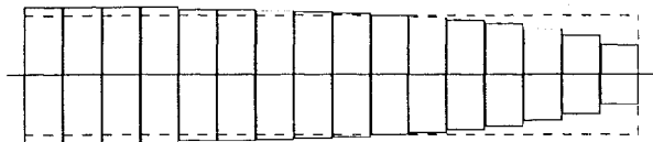
Fig. 7 Searched shape ( d_i/d_0 ) of column, C/F condition.
